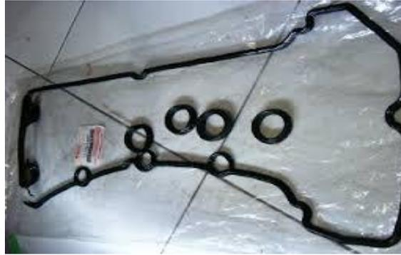
Gambar 3.1. *Packing oil seal* mesin mobil
